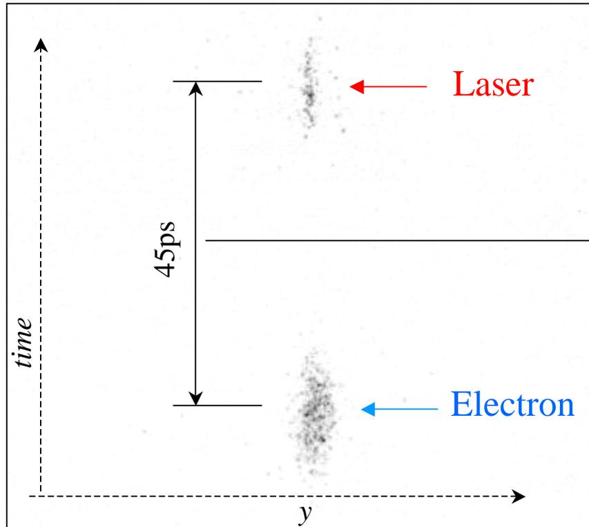
Delay introduced by the presence of the doubling crystal
