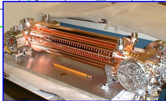
0.6-m section, 22 MV available at SLAC (200- $\mu$ m alignment)
