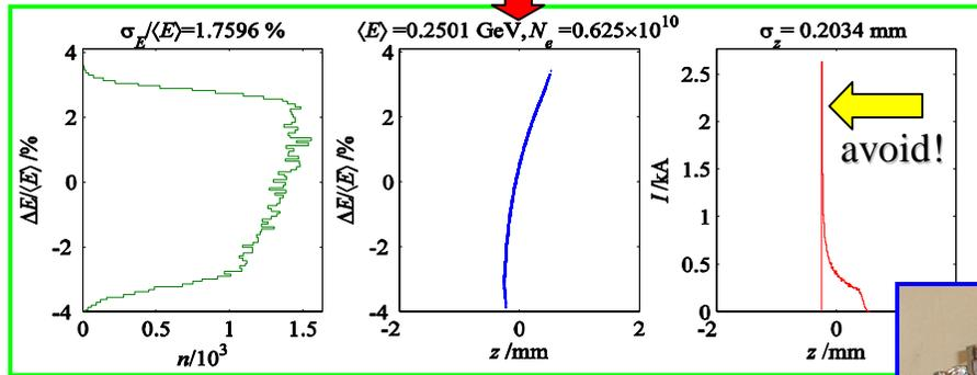
X-band RF at decelerating phase corrects 2<sup>nd</sup>-order and allows unchanged  $z$ -distribution
