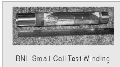
BNL Small Coil Test Winding
