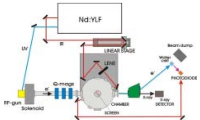
Figure 3: Beam line layout for X-ray generation experiment.
