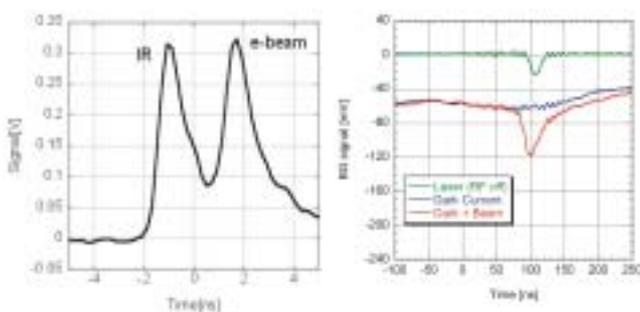
Figure 5: Typical scope-trace of photodiode output shows the electron beam signal (Cherenkov light) and IR laser light (left). Background signal of X-ray detector (right)
