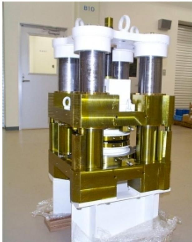
Fig. 1 1/3 scale model of permanent magnet for 3 MeV cyclotron.
