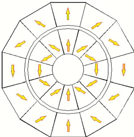
Fig. 8 Cross section of Two layer Halbach type dipole magnet.
