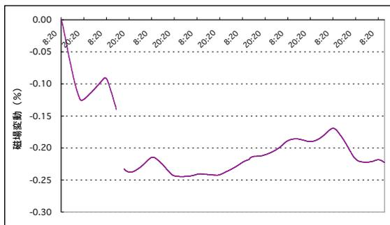
Fig. 3 Magnetic field variation of magnet.
