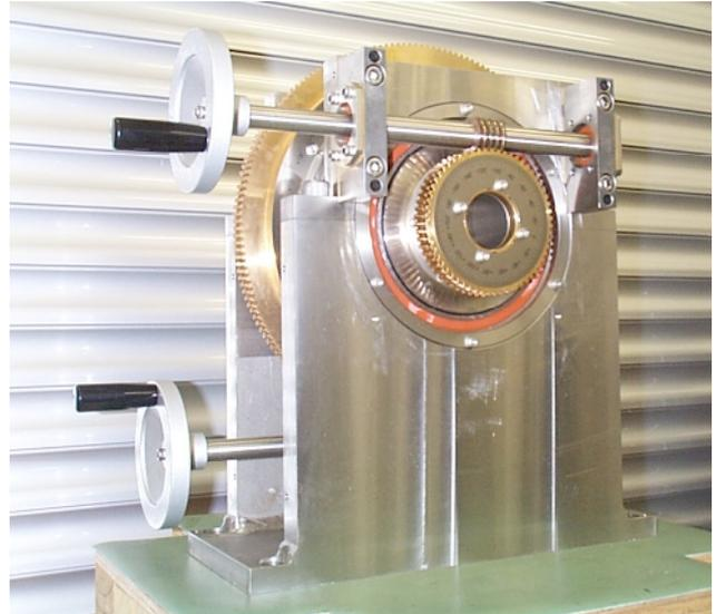
Fig. 9 Photos of Two layer variable field Halbach type dipole magnet. The normal field strength could be changed without introducing skew component.
