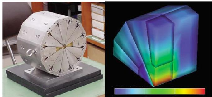
Fig. 10 4.45T magnet (at  $-29^{\circ}\text{C}$ ). The magnetic field at room temperature is 3.9T.
