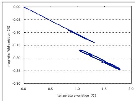
Fig. 4 Magnetic field vs. magnet temperature.
