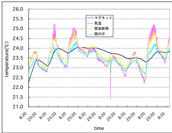
Fig. 2 Temperature variation of magnet, ambient temperature, insulated box A, insulated box B. Insulator was not installed on the first day.
