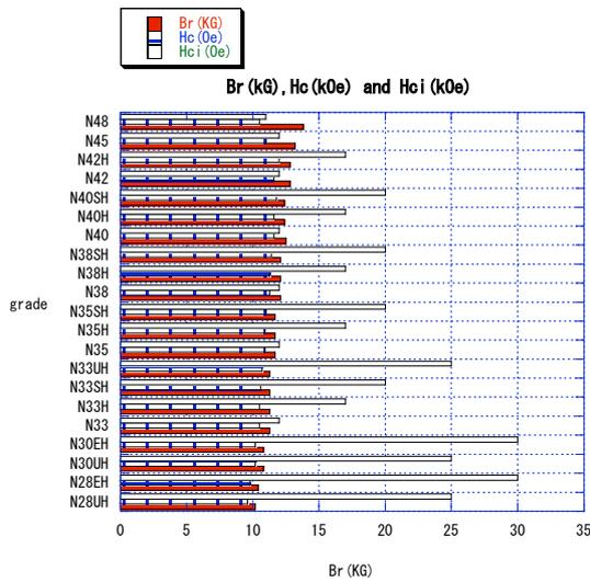
Fig. 7 Intrinsic coercive  $H_{ci}$  (green diamond), coercive force  $H_c$ (red circle) and residual field  $B_r$ (blue rectangle).
