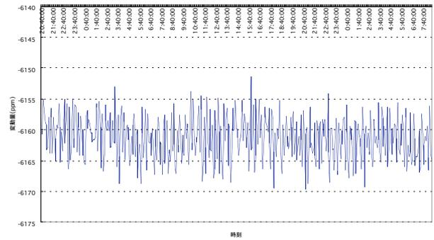
Fig. 5 Magnetic field variation vs. time. Vertical axis denotes field variation and horizontal axis denotes elapsed time. One division in vertical axis corresponds to 5 ppm.
