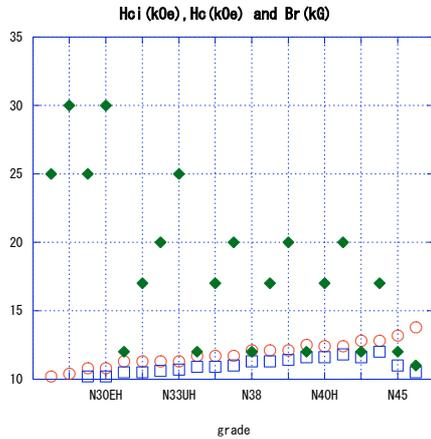
Fig. 6 Intrinsic coercive  $H_{ci}$  (green diamond), coercive force  $H_c$ (red circle) and residual field  $B_r$  (blue rectangle). Intrinsic coercive  $H_{ci}$  varies in a wide range for each material of the same energy product.
