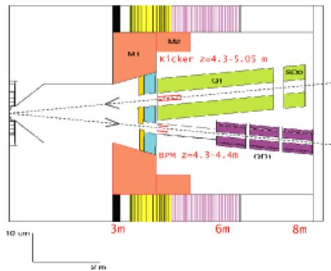
Figure 2: GEANT model of NLC IR showing the positioning of the IP feedback kicker and BPM components.
