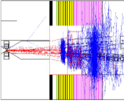
Figure 3: GEANT model of NLC IR with 20 tracked  $e^+e^-$  background pairs. The scattered and secondary charged particles are shown in red and neutral photons in blue.
