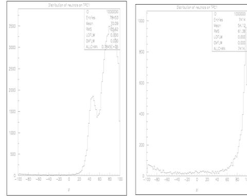
Figure 9: Distribution of background photon flux in the TPC for the 'near' and 'far' feedback configurations.
