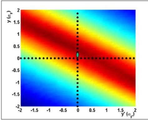
Figure 11: Luminosity of test 2 bunch banana bunch collision with varying  $\Delta y, y'$  offsets.
