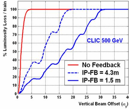
Figure 7: Simulation of luminosity loss at CLIC 500 GeV machine with varying initial beam offsets at the IP.
