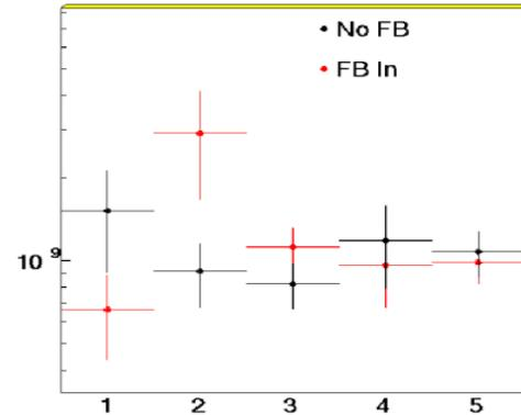
Figure 6: The neutron flux in the 5 layers of the vertex tracker with and without the feedback system included in the IR FLUKA99 model.
