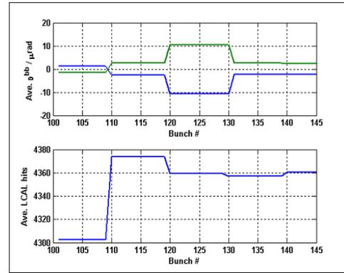
Figure 13: The beam-beam kick (proportional to IP FB BPM reading) for bunches 100-150 demonstrating the luminosity feedback system in operation. The bottom plot shows the luminosity monitor signal ( $e^+e^-$  pairs hitting LCAL). Note the integration over 10 bunches per signal.
