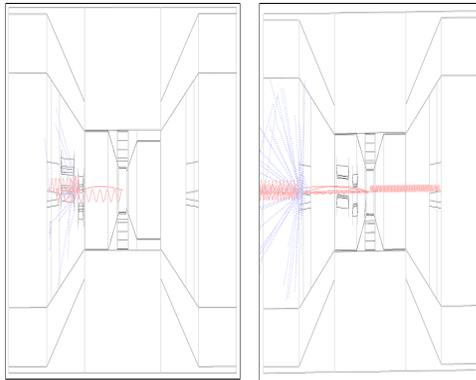
Figure 8: The CLIC IR geometry with 2 feedback configurations: 'near' (right) and 'far' (left).
