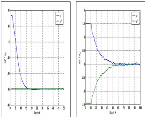
Figure 12: IP  $y$  and  $y'$  bunch positions at the IP for the first 100 bunches in the train with the fast feedback system operational.
