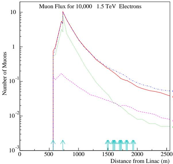
Figure 8: Muon flux determination from Geant4 for a 1.5 TeV beam with a -2% offset in energy. The positions of the spoilers and collimators are shown by arrows. Case *a* corresponds to magnet elements consisting of unmagnetised (and case *d* magnetised) cylinders of iron of diameter 20 cm with fully simulated showers. Case *b* is as case *a* except that only the first photon of a shower contributes. Case *c* is the same as case *a* except the magnet elements have diameter 50 cm.
