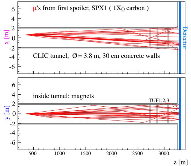
Figure 1: Tracking of muons, produced at the first spoiler, through the beam delivery system up to the detector region. Top is the horizontal and bottom the vertical plane.
