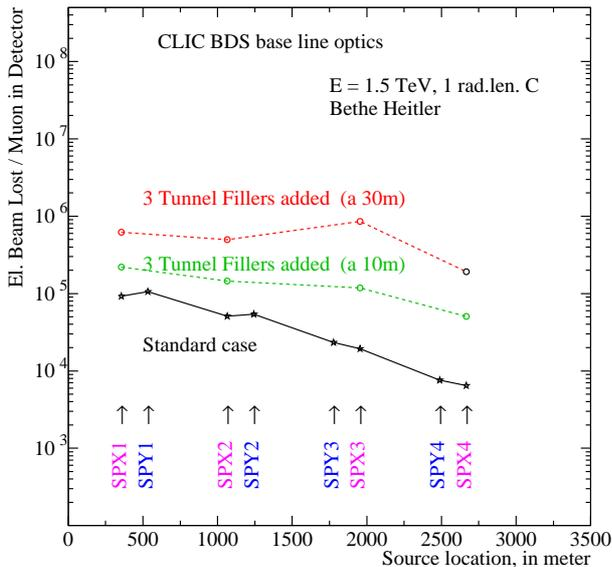
Figure 3: Number of lost electrons per muon passing through a detector with 7.5 m radius as a function of position along the baseline final focus. Potential collimator locations are indicated. The IP is at 3282 m.
