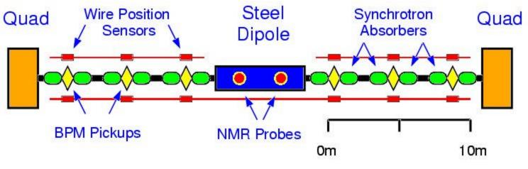
$E \propto \frac{1}{\theta} \int BdI$  - Only a relative energy measurement - Dipole mapped at many energies
