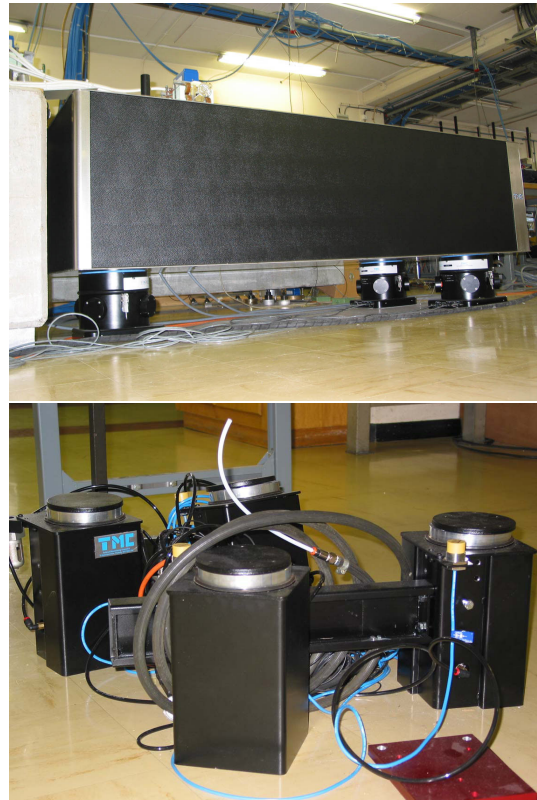
Figure 4: Top: Picture of the honeycomb table supported by three feet that perform vibration damping. Bottom: The alternative pneumatic system for passive and active vibration damping and micron alignment. It can be mounted below the honeycomb table.
