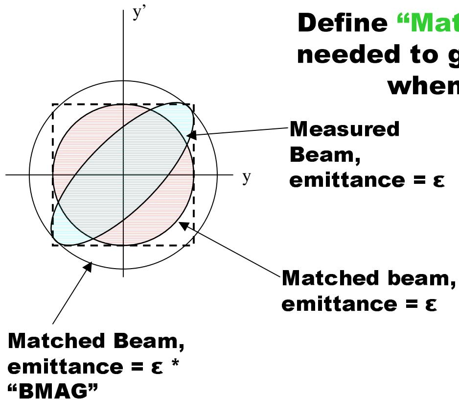
**Define “Matched”  $\equiv$  “Has the parameters needed to give me the design value of  $\beta^*$  when transported to the IP”**
