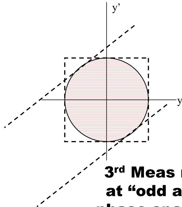
**3<sup>rd</sup> Meas must be at “odd angle” in phase space (not 0 or 90 degrees)**
