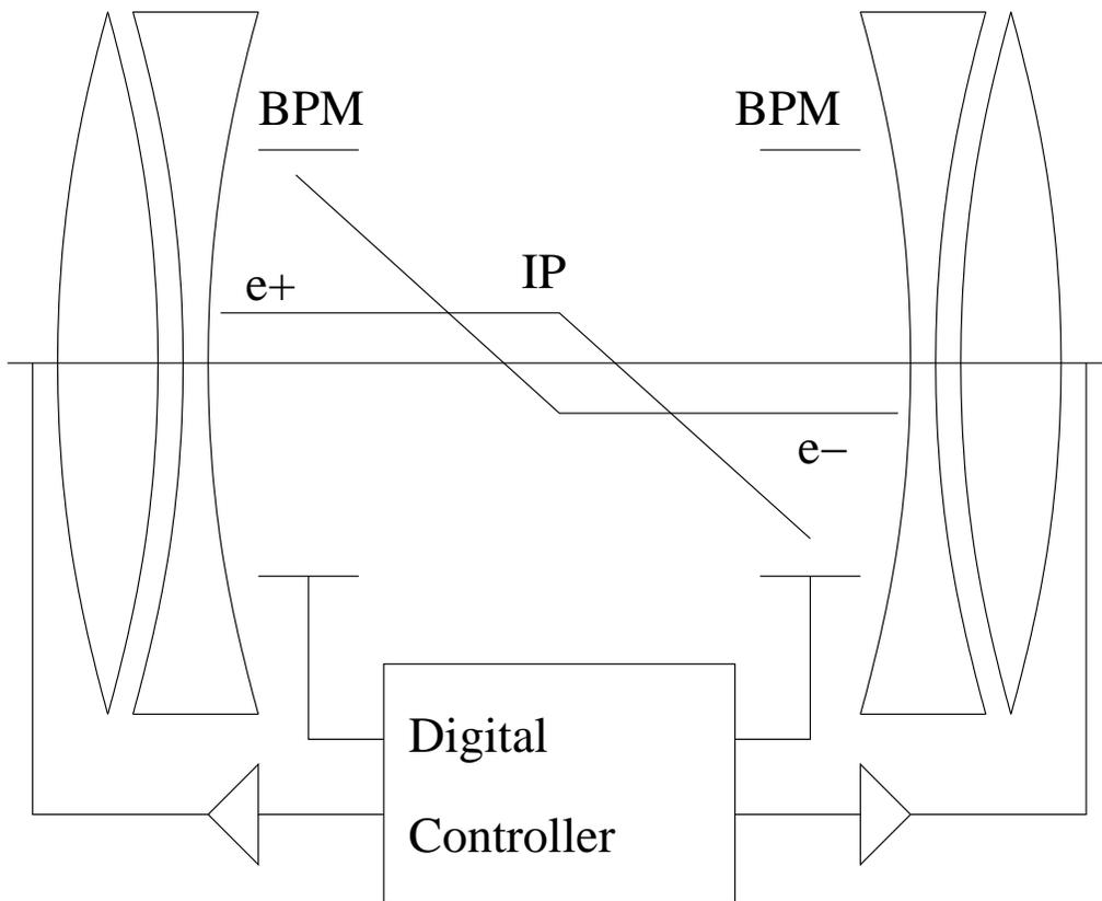
Infer beam offset from beam-beam deflection.
