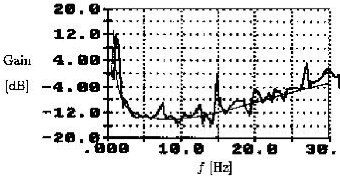
Measured rms vibration amplitude on the floor and on the magnet:
