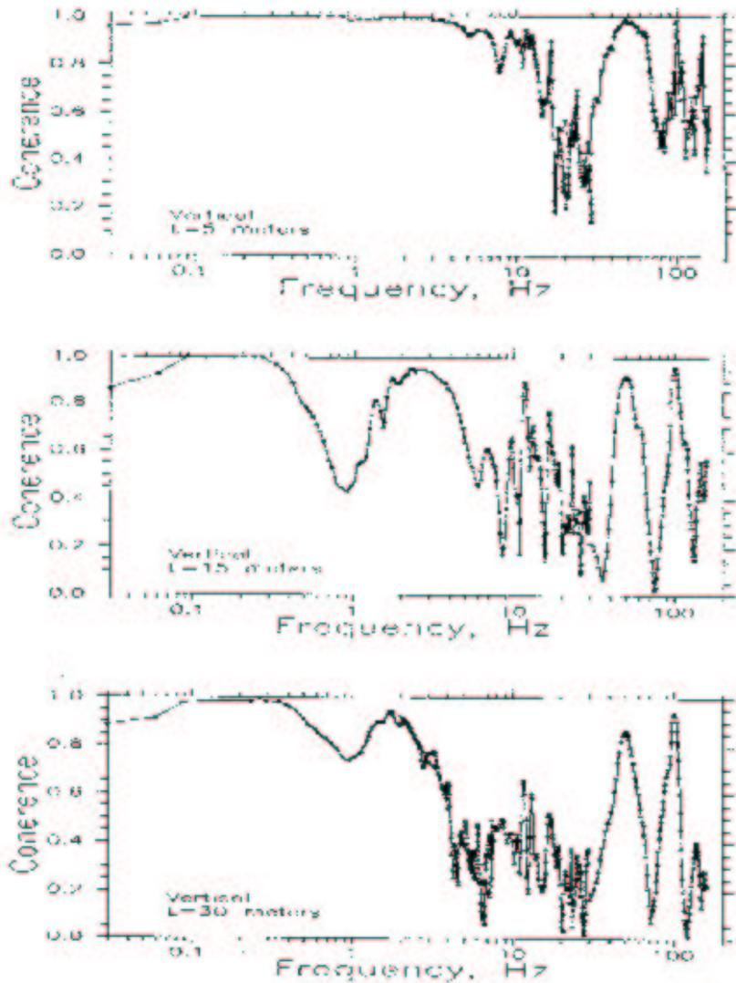
→ Quadrupole motion in SBLC will be uncorrelated for frequencies above 2 Hz.
