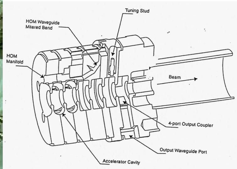
Inner surface accurate to  $1\mu\text{m}$
