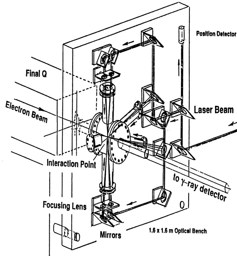
Succeeded in measuring **50nm** beam at FFTB
