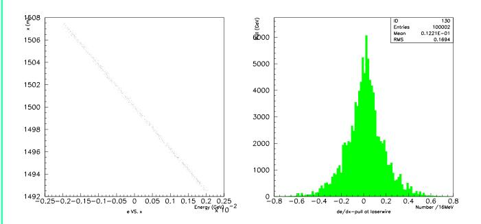
Intrinsic resolution  $\sim$  170 MeV. Matching this to the spotsize measurement requires endpoints of x-distribution to be determined to within 45  $\mu \rm m$ .  $\Longrightarrow$  Should be possible to obtain energy-spread measurement to  $\sim 10^{-4}$
