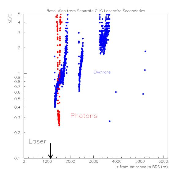
$\longrightarrow$  At best a 25% measurement using photons. Electrons are harder because they are more spread out by magnetic fields.
