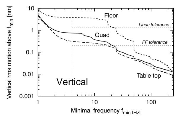
On magnet top: X:  $(0.4 \pm 0.1)$  nm Y:  $(0.9 \pm 0.1)$  nm (0.3 nm on table top) Z:  $(3.2 \pm 0.4)$  nm
