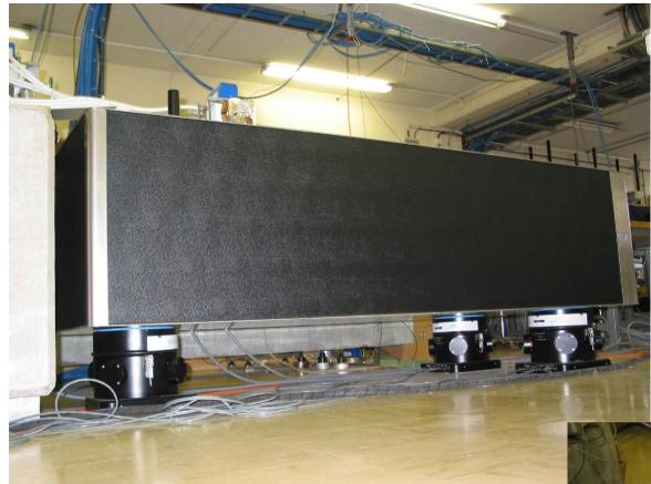
STACIS 2000 (TMC) Rubber damping Active feedback circuit on ground motion Measure ground motion Actuators: piezos
