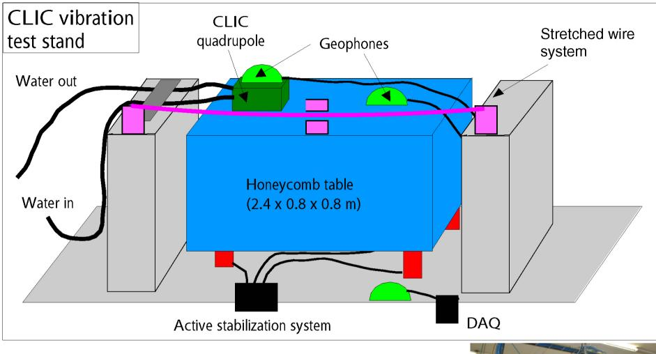
Vibration damping: Cooling water: Vibration: Alignment: Support platform: Two systems (rigid or soft) on/off Geophones Stretched wire system Lowest resonant frequency > 230 Hz
