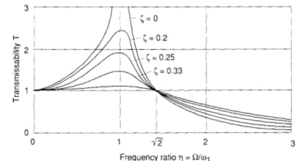
Transmissibility of an isolator as a function of frequency ratio
