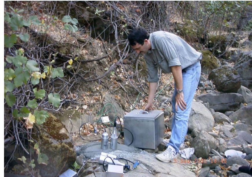
**Probes were placed on the concrete bed at the measuring spot, then they were covered with a shielding enclosure.**
