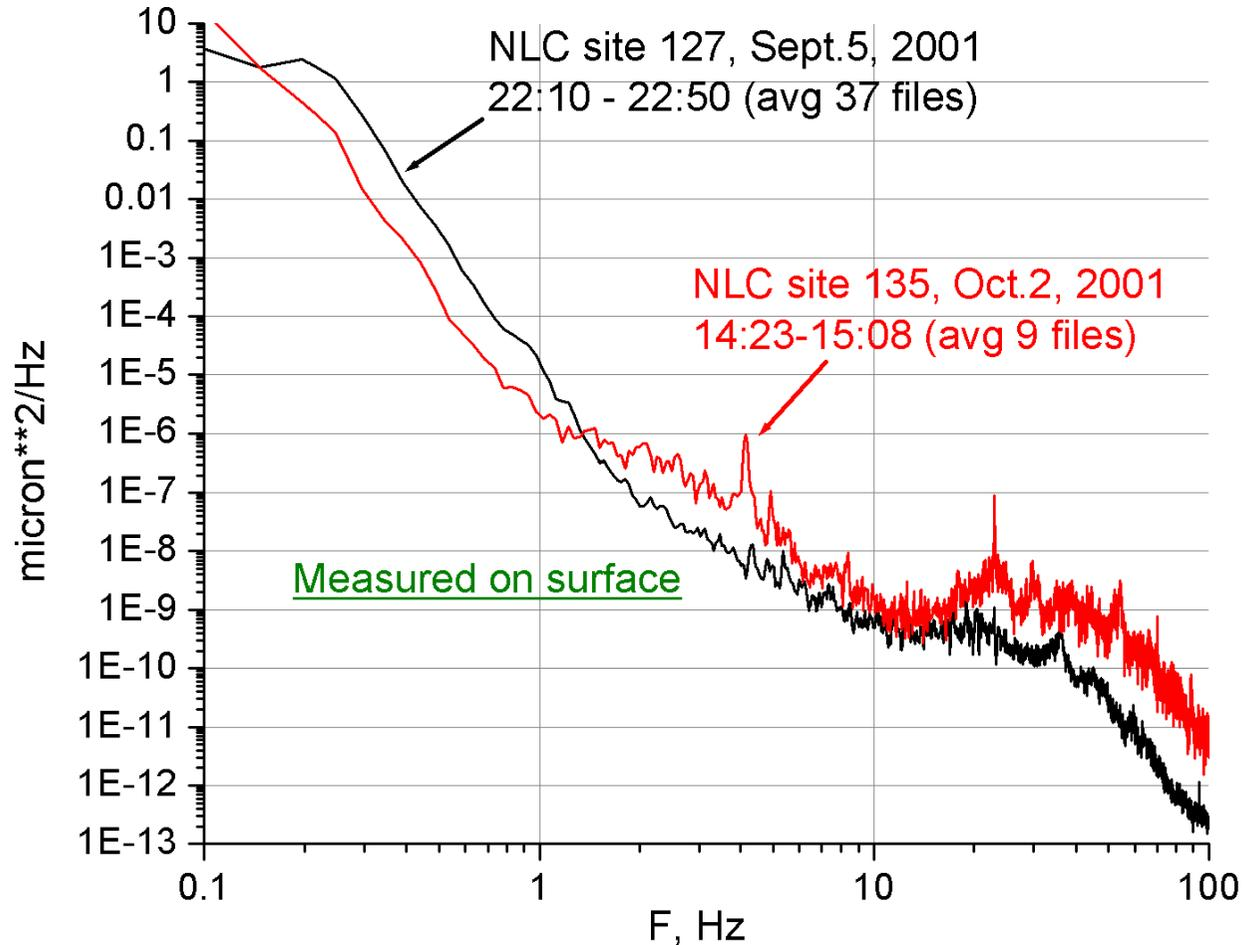
**Power displacement spectrum measured at the west spot at site –135-E ,
