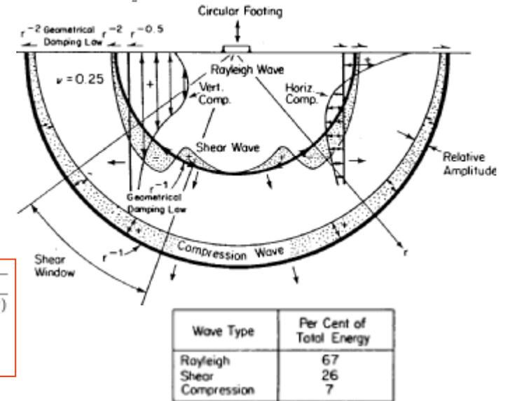
Figure 3-16. Distribution of displacement waves from a circular footing on a homogeneous, isotropic, elastic half-space (from Woods, 1968).
