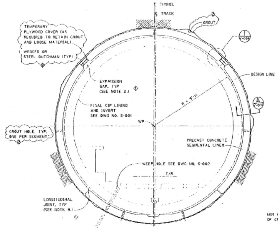
Typical Cross-Section of the MTA Tunnel
