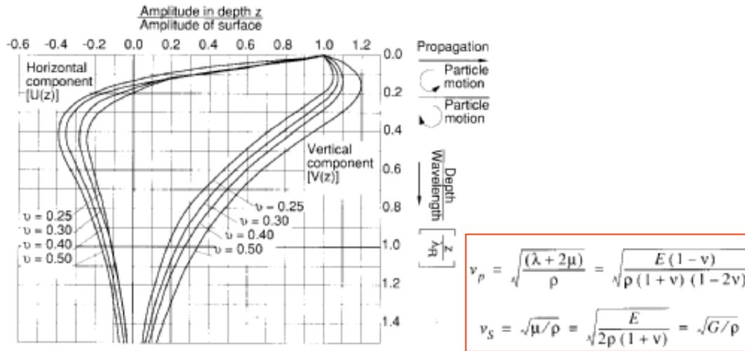
Figure E.2: Relation between amplitude ratio and dimensionless depth for Rayleigh waves with  $\nu$  as parameter
