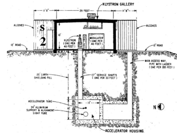
Typical Cross Section of Accelerator Housing and Klystron Gallery at SLAC
