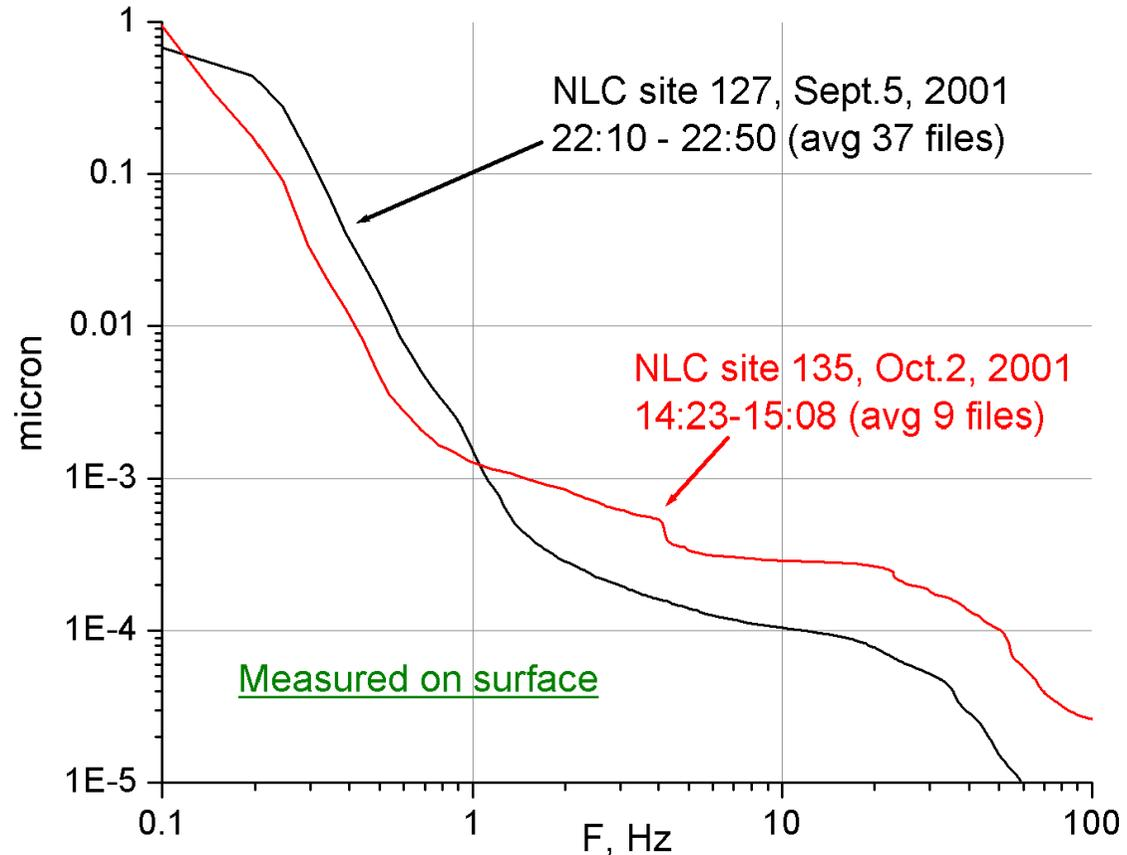
**Displacement spectrum measured at the west spot at site –135-E , as compared with data from site-127**
