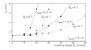
Figure 4: Simulated vertical spot size  $\sigma_y^*$  at the CLIC collision point vs.  $\theta_c$  considering solenoid fields of 4 and 6 T [9].
