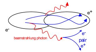
Figure 9: Ilustration of beam-beam phenomena in a linear collider: beamstrahlung and pair production during the collision of electron and positron bunches.
