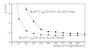
Figure 5: Simulated vertical spot size  $\sigma_y^*$  at the CLIC collision point vs. length of the fringe field (right), considering solenoid fields of 4 and 6 T [9].
