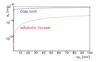
Figure 7: Miminimum IP spot size  $\sigma_{y_{\min,AF}}^*$ , Eq. (18), as a function of the normalized emittance.
