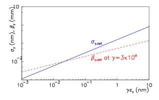
Figure 3: Miminimum IP spot size  $\sigma_{y_{\min}}^*$ , Eq. (11), as a function of the normalized emittance, assuming  $F \approx 5.4$ .
