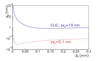
Figure 2: Vertical IP spot size  $\sigma_y^*$ , Eq. (8), as a function of the IP beta function, for a normalized emittance of 10 nm, and a 100 times smaller emittance, and assuming  $F \approx 5.4$  (value for the CLIC final focus).
