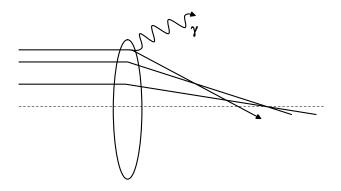
Figure 1: Schematic of Oide effect; particles emitting synchortron radiation in the final quadrupole are no longer focused at the collision point.
