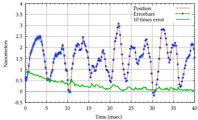
Figure 10: Interferometer Position and Error vs Time
