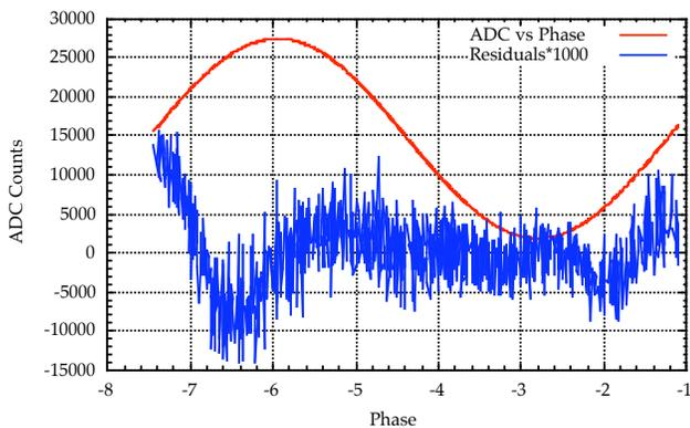
Figure 9: Photodiode Voltage vs Fitted Phase and Residuals multiplied by 1000
