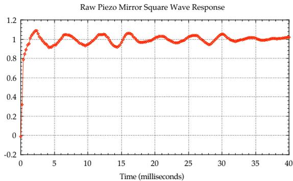
Figure 12: Measured Step Response of Piezo Mirror
