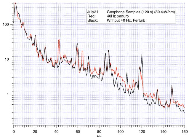
Figure 2: Vertical Ground Motion Amplitude (nm) vs Frequency in UBC Physics Basement
