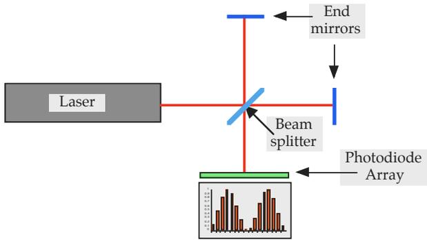
Figure 7: Michelson Interferometer
