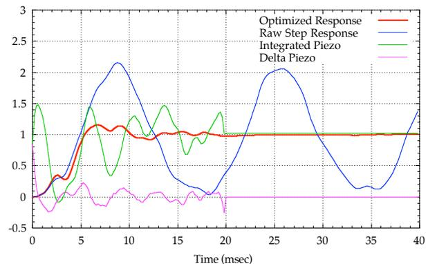
Figure 6: Calculated Optimal Piezo Sequence and Calculated Platform Response
