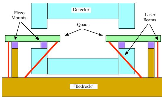
Figure 1: Optical Anchor concept
