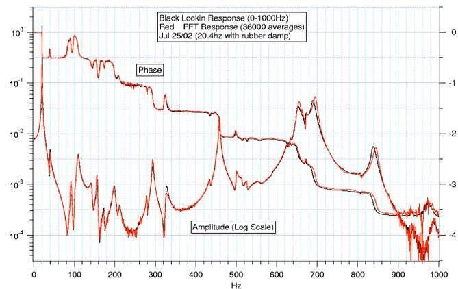
Figure 4: Platform Response to Piezo vs Frequency (log amplitude, cycles of phase vs Hz)
